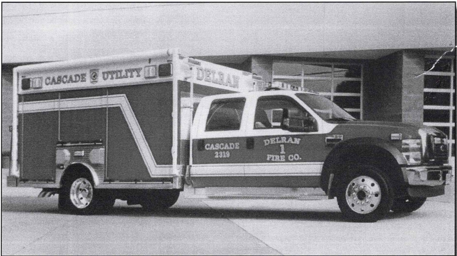
2009 Ford F-550 Cascade / Utility Unit. Hi-Pressure Cascade with a booster pump. This truck replaced our 1986 Chevrolet Van.
