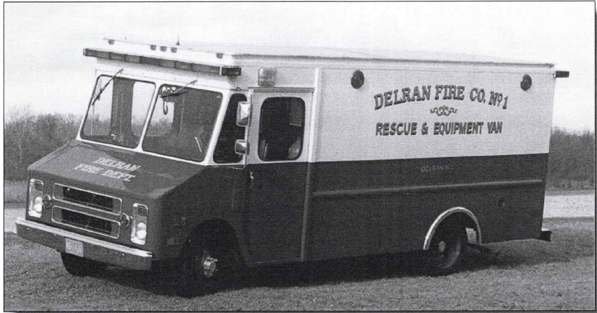
1986 Chevrolet (Grumman) Rescue and Equipment Van. It had a diesel engine, automatic transmission and was equipped with a six bottle, 6000 psi cascade system.
